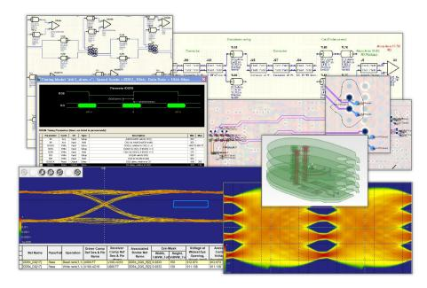
HyperLynx SI supports pre- and post-layout signal integrity, timing, crosstalk, and power-aware simulation. Automated workflows support complete interface-level DDRx verification and compliance analysis of standards-based SerDes channel designs.
